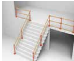
ANGLED STAIR WITH TWO-SIDED OPENING
